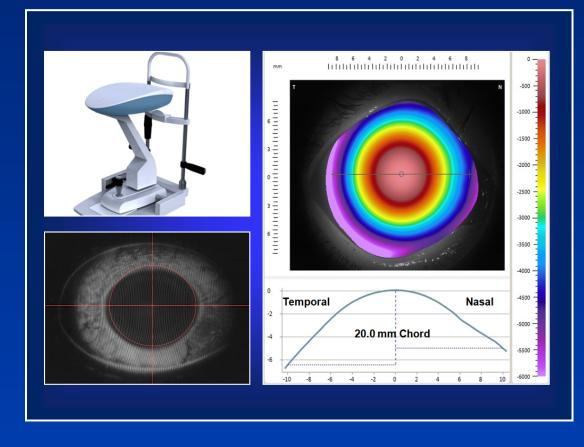
The Eaglet Eye Surface Profiler uses a double projection infrared, moiré profilometer to capture the surface profile of both the cornea and the sclera. The ESP can measure diameters of up to 20mm, 360 degrees around. With more than 250,000 data points, it directly measures corneal and scleral height to produce highly accurate elevation profiles and maps.
